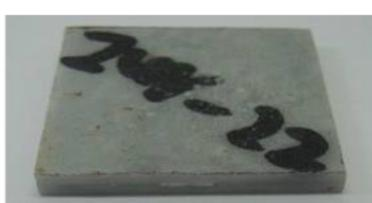
Fig 5a: 2-layer UV cured sample after 312 hours seawater exposure after 312 hours seawater exposure
